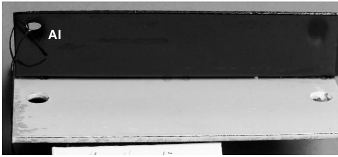
Figure 6. Hybrid sample with coating system 2 after 30 cycles acc. to PV 1210
